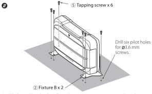
Drill the pilot holes for  $\phi$ 3.6 mm screws on the sheet metal section of the vehicle, and attach the speaker unit to the vehicle using the tapping screws (5).
